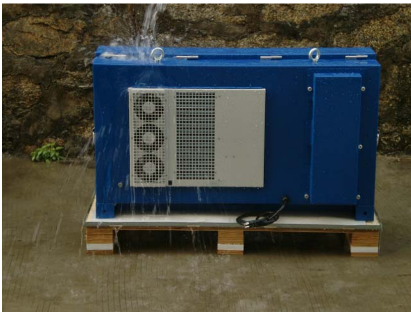
Waterproof testing in progress
